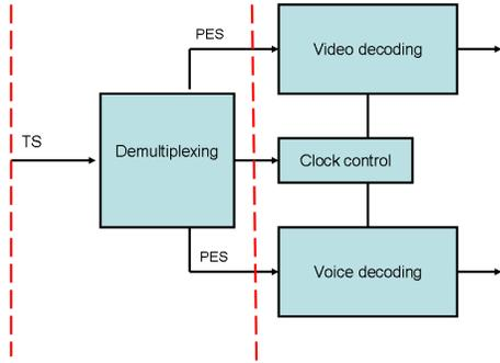
Fig. 3. Decoding process of TS.
