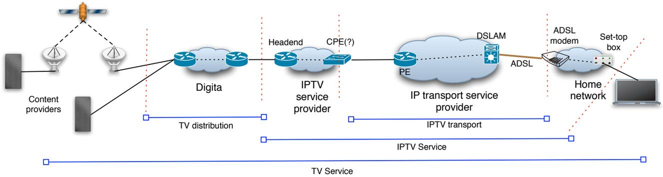
Fig. 1. A real-world example of multicast based IPTV delivery.
